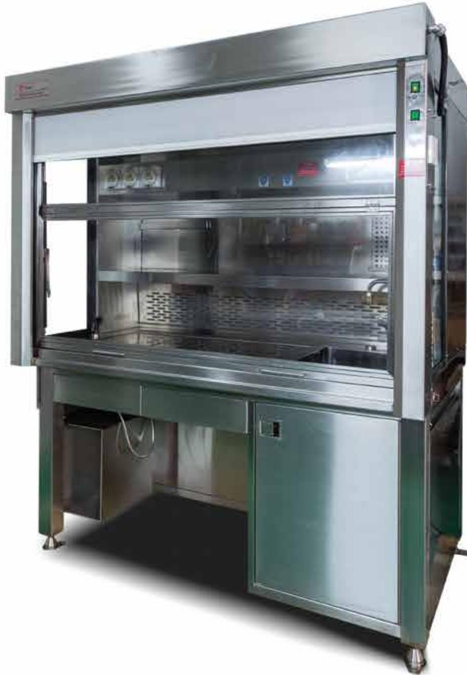
The B-Series grossing workstation provides special features to allow grossing of fresh & potentially infectious samples. Features include HEPA filtered exhaust to capture infectious particles, height adjustable splash shield & UVC light for surface decontamination after grossing together with UVC shield to protect users from the UVC radiation.
